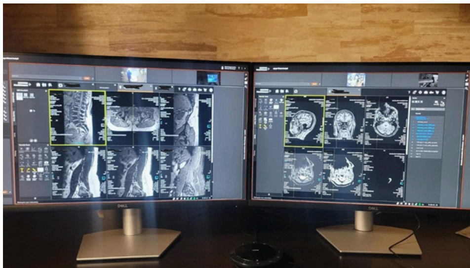
Figure 2: SVC workstation demonstrating two units/patients being scanned remotely. Note at the center top of each screen is the camera pointed down the bore of the magnet. The second camera in the upper right corner is pointed towards the power injector. On the counter between both monitors is the microphone/speaker for communicating with the tech assistant.
